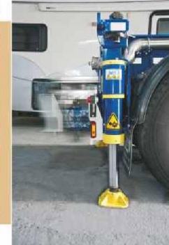
For ergonomic usage partial rear underrun protection device which is extended by hydraulic cylinder
