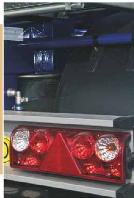
Lighting system according to ECE R48
