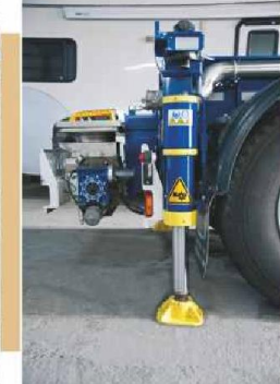
For ergonomic usage partial rear underrun protection device which is extended by hydraulic cylinder
