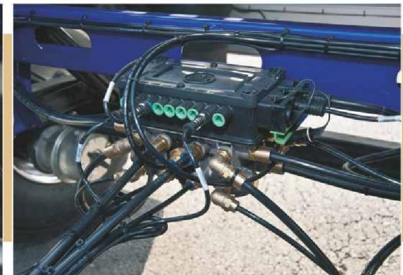
Alternative brake circuits equipped with EBS according to R13
