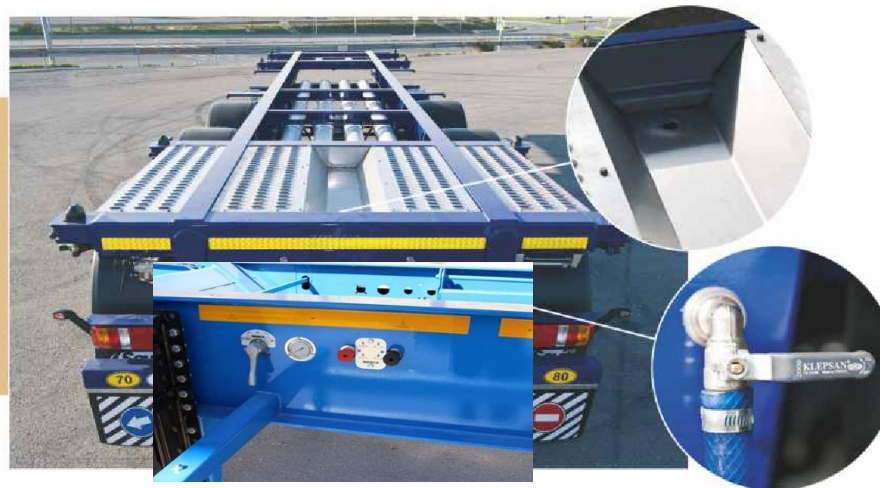
Stainless steel drainage, pool, aluminium walkway and valve for chemicals to avoid pollution
