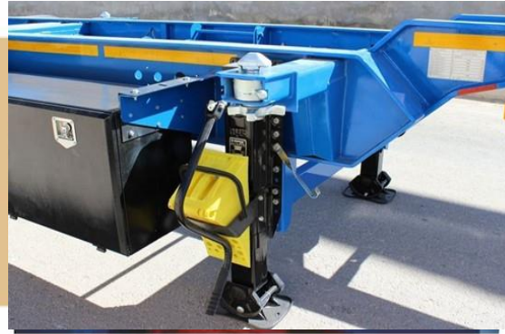
Front container twistlock and extending rear bumper for carrying 45 ft container
