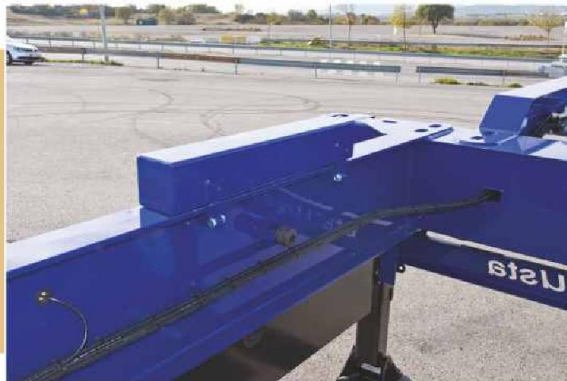
Folding container supports for to carry containers without tunnel
