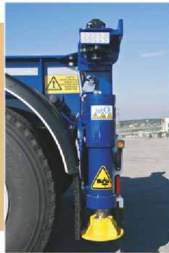
By the rear connection, 24 V DC controller to power the features of semi trailer
