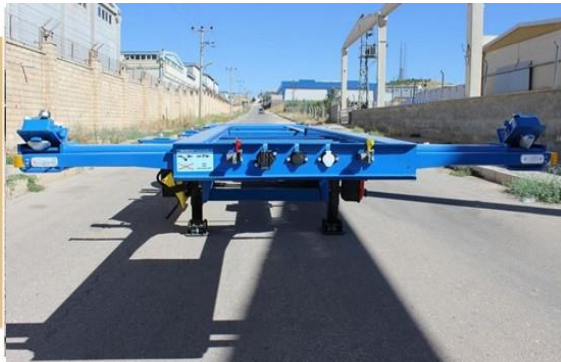
Rear hydraulic support legs to provide secure operation on different ground conditions
