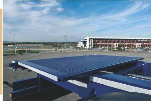
Adjustable rear ramp for easy unloading 20 ft
