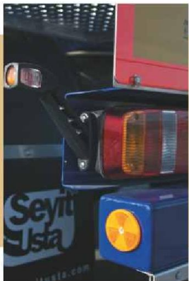
Lighting system according to ECE R48
