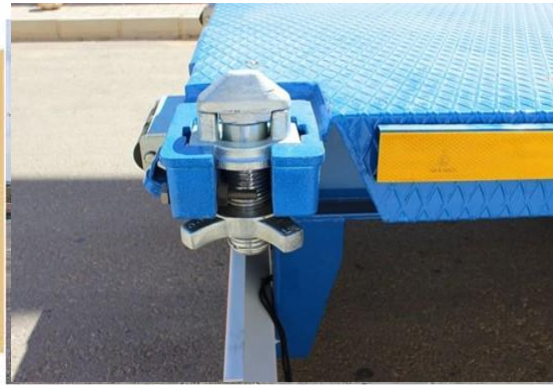
Front container twistlock and extending rear bumper for carrying 45 ft container
