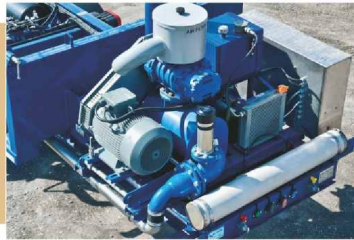
Low decibel blower to generate air pressure to pump granules to the silos powered by an electrical engine (optional diesel engine)
