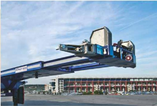
Front container twistlock and extending rear bumper for carrying 45 ft container
