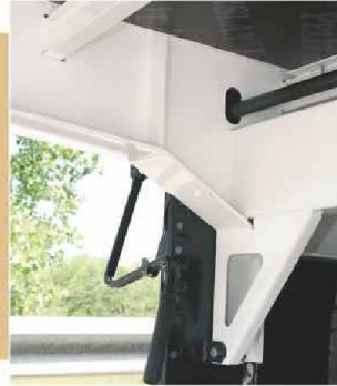
Light chassis produced from quenched steel for more payload.
