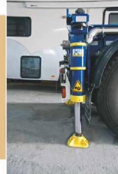
For ergonomic usage partial rear underrun protection device which is extended by hydraulic cylinder
