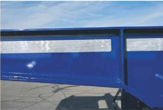
Light and strong chassis made of high strength steel for more payload
