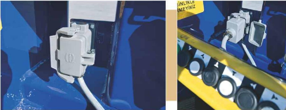
By the rear connection, 24 V DC controller to power the features of semi trailer
