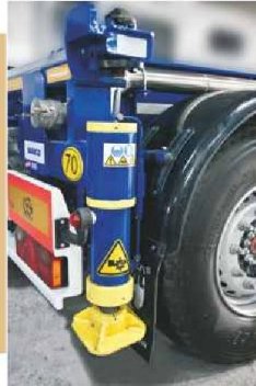
Rear hydraulic support legs to provide secure operation on different ground conditions
