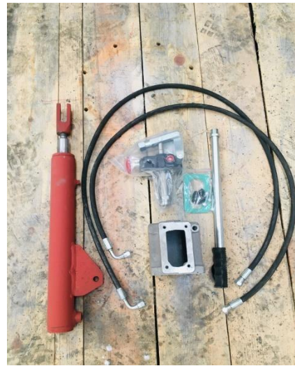
Discharge Chute Lifting Jack
