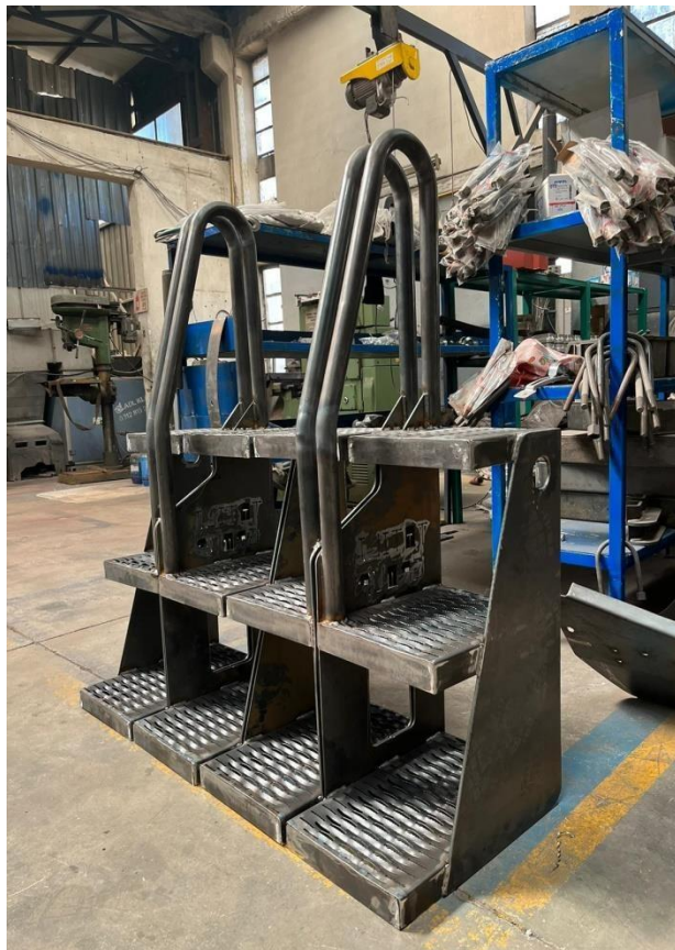
Concrete Pump ladder
